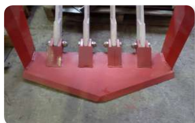
Anti-wear steel tip
