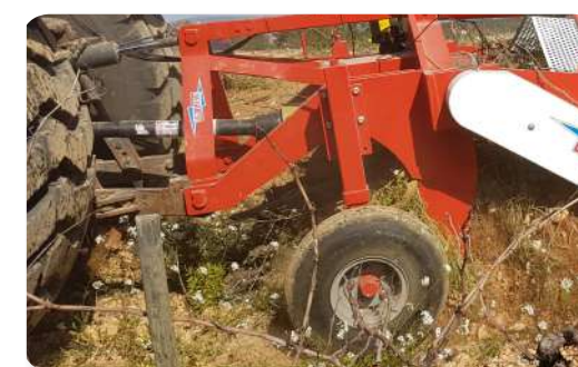
Pneumatic tyres for depth control
