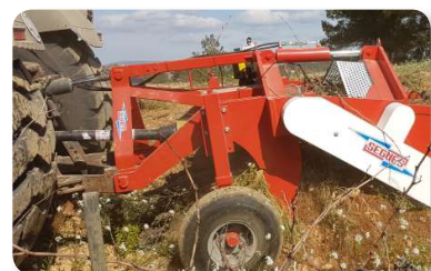
Hitch with the third point CAT-III
