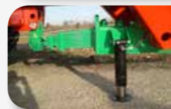
Mechanical jack in RA-TM10 & 15 and hydraulic jack in RA-TM20
