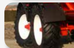
Tandem and self-steering axle in RA-TM15 & 20
